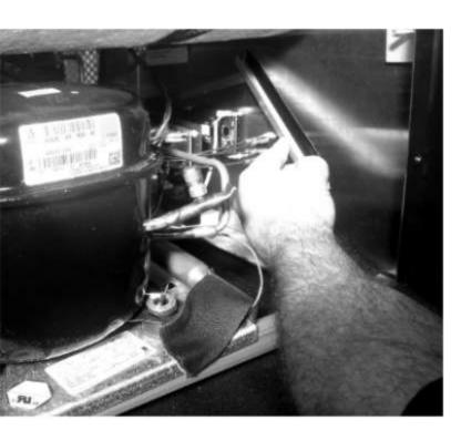
Place the gutter a little past the lowest point on the chamber.
