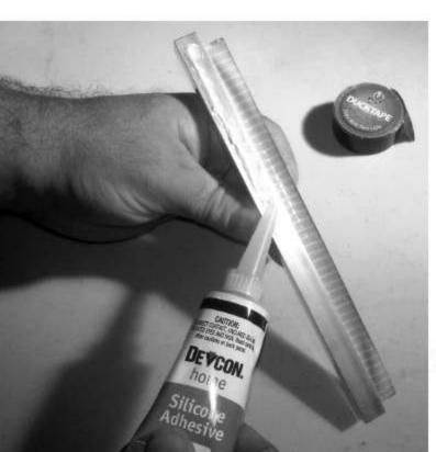
2. Apply silicone to gutter.
