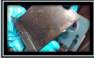
Rusted Splash Guard
